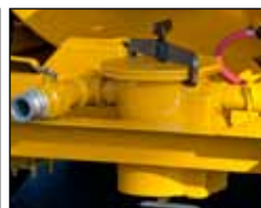
2.5 gallon material filter for extended spray periods
