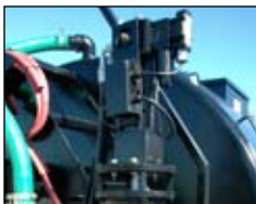
ESSP hydraulic piston pump w/ Generation III pump head
